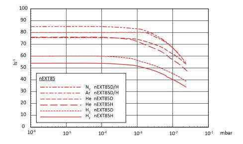
Figure 14 nEXT85 pumping speed versus inlet pressure performance graph
