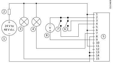
Figure 20 Logic interface connections - parallel control
